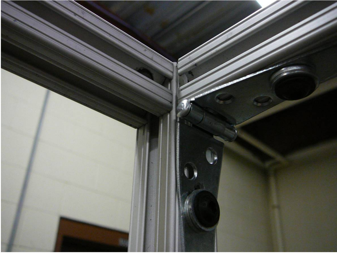
Close-up view of hinge mechanism in top corner of frame. One dimension folds for storage, the other remains fixed.
