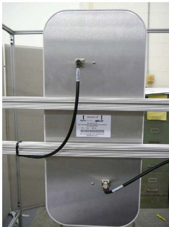
The antenna (rear) as mounted to test apparatus frame showing connections to PC and tag reader.
