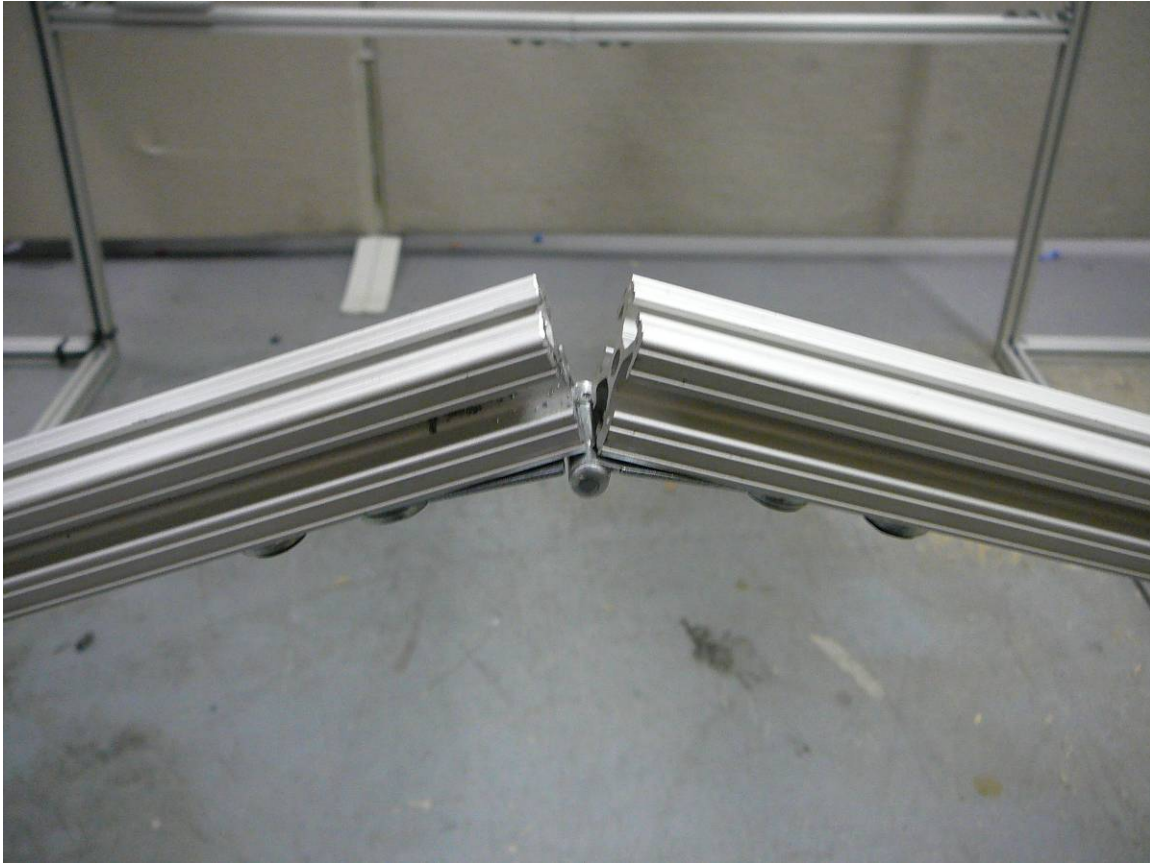
Close-up view of galvanized steel hinge mount on test apparatus, for collapsibility and easy storage.
