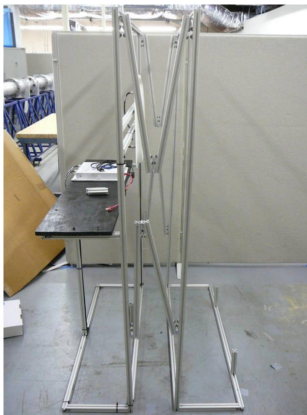
Test apparatus in collapsed form, showing galvanized steel hinge mechanisms and reduced floor footprint.
