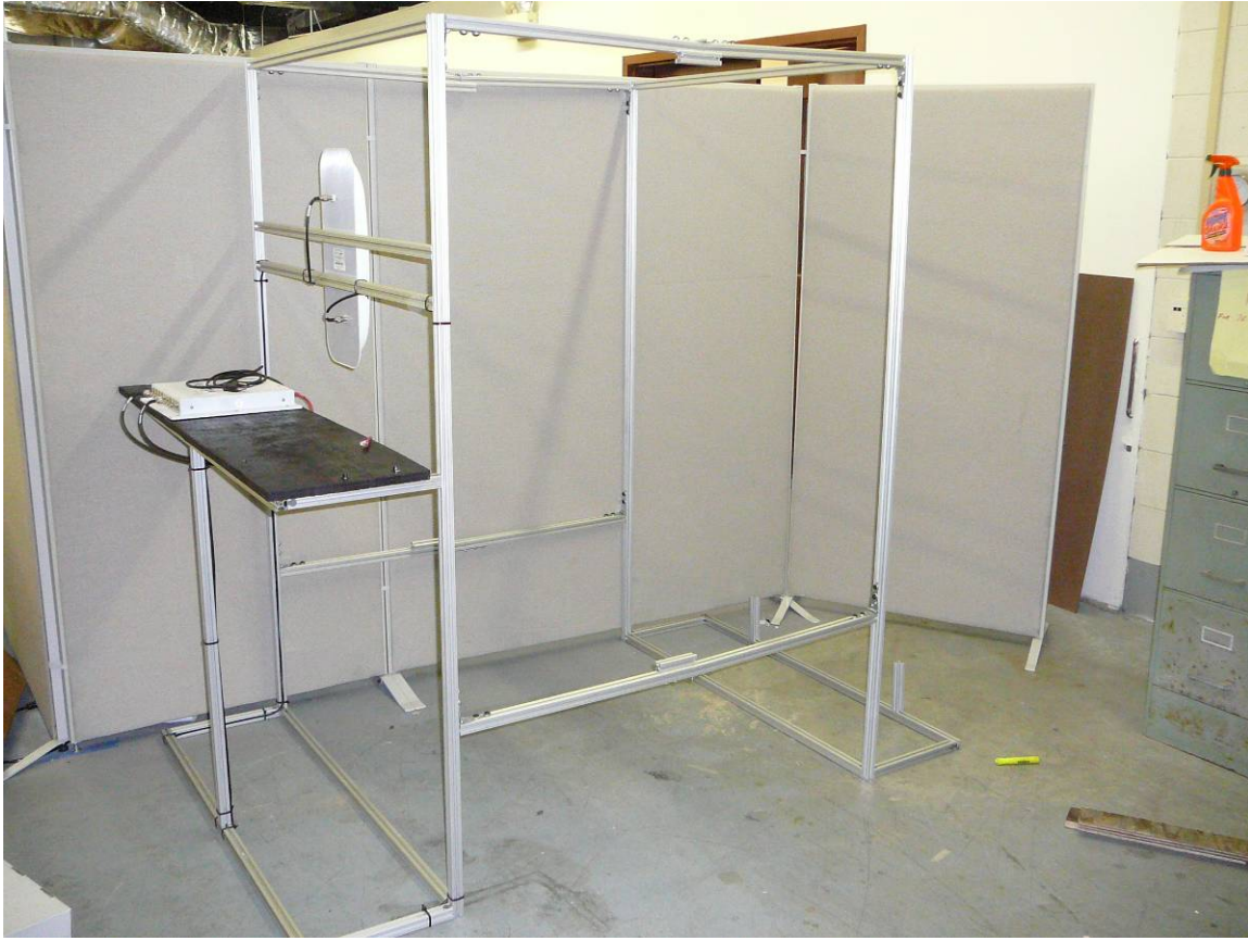
Test apparatus in expanded form, showing collapsible T6105-T5 Aluminum extruded frame and steel hinges, antenna, and support shelf for PC and ThingMagic reader.
