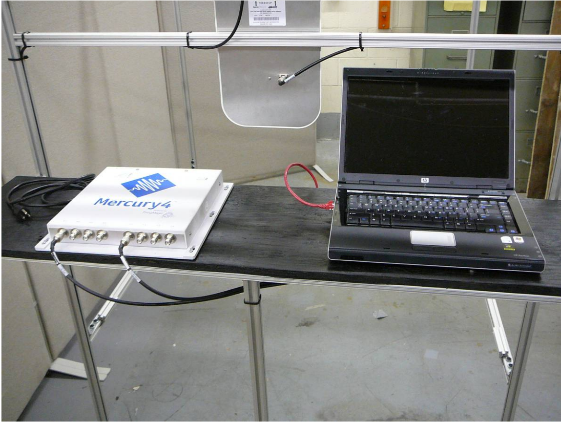
Test bench setup with ThingMagic tag reader and a PC for data acquisition and analysis through MATLAB.
