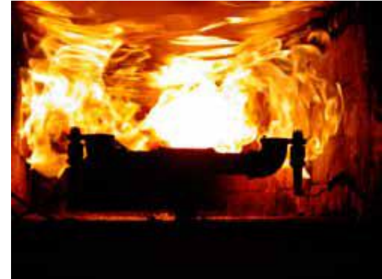
Fire test tunnel 1860° F
